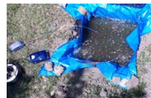
Gambar -9 : Oxidation Pond Skala Laboratorium
